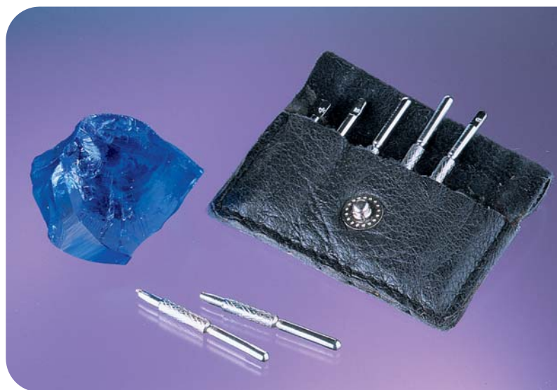
Figure 24. As a last resort, a portable hardness testing kit (here, 6.5 × 4.0 cm) can aid in identifying rough when visual testing is reduced due to a rough surface or natural tumbling. Hardness testing should not be done on fashioned gems. Photo by Maha Tannous.
