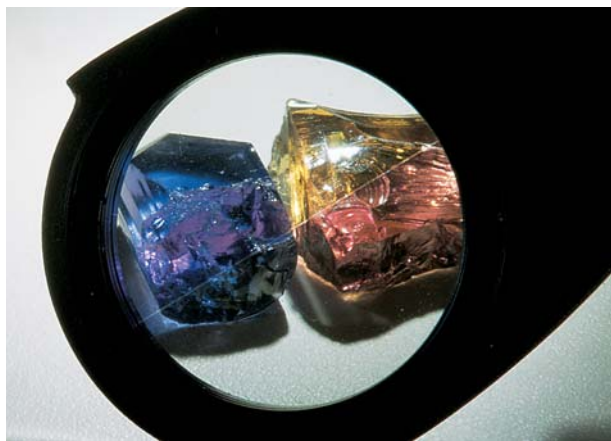
Figure 15. The new London Dichroscope, distributed by the Gemmological Association of Great Britain, has an expanded field of vision that makes it ideal for viewing larger gems or rough, such as this tanzanite (left, 2.57 grams) and pink zoisite (right, 2.9 grams). Stones courtesy of H. Krupp; photo by Maha Tannous.
