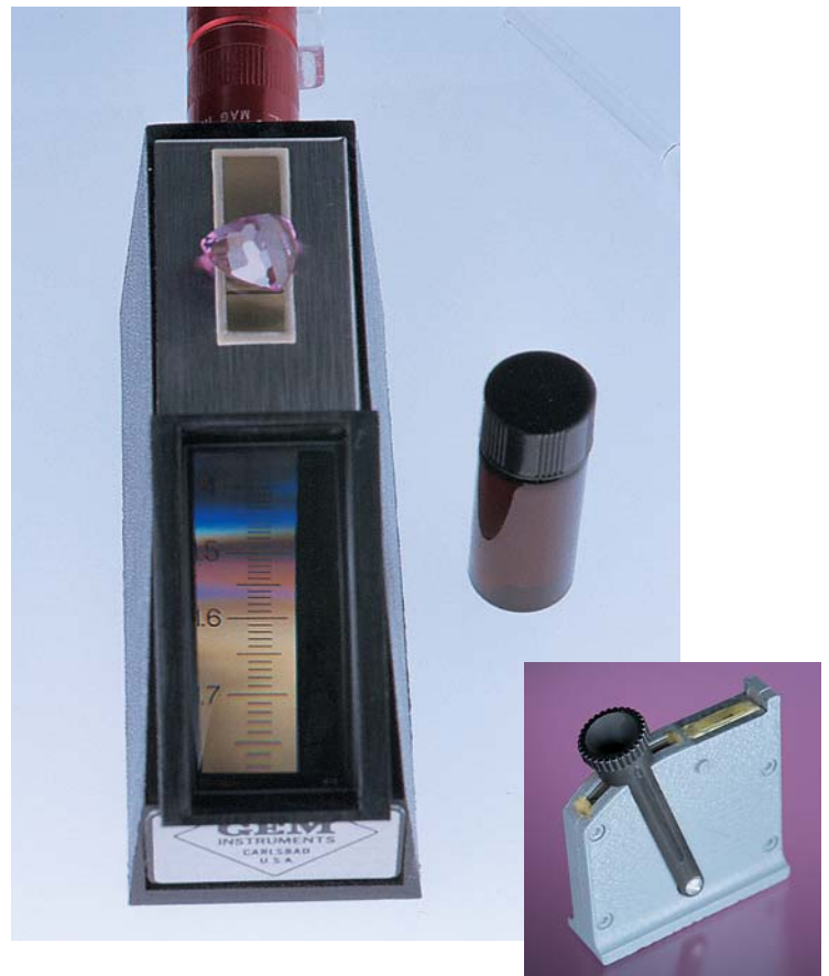
Figure 20. Among the portable refractometers currently available is the GIA Gem Instruments Duplex III (shown with a 4.95 ct spinel). The inset shows the GIA Gem Instruments refractometer designed by Robert Shipley Jr. that was introduced in 1949. At 5.2 × 4.8 cm, it is still considered one of the most durable and portable refractometers ever made (E. Gübelin, pers. comm., 2002). Photos by Maha Tannous.
